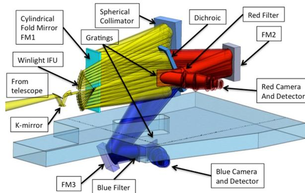
KCWI Isometric Opto-Mechanical Layout (KCRM is the Red Optical Design in the Schematic)
