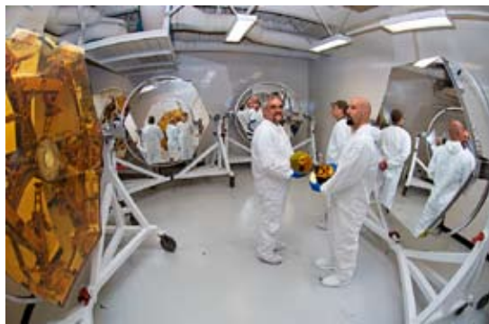
Above: Individual mirror segments are cleaned and re-coated to optimize telescope performance. Top right: MOSFIRE undergoes final testing at temperatures close to absolute zero. Bottom right: Upgrades will deliver greater sensitivity and stability to Keck's most in demand spectrograph, LRIS.
