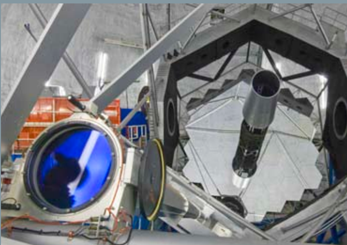
Keck II laser launch tube positioned next to the primary mirror.
