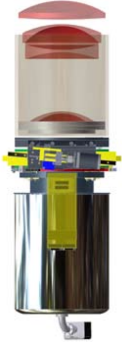
Model of the enhanced dewar and focus mechanism for the LRIS red channel detector upgrade.
